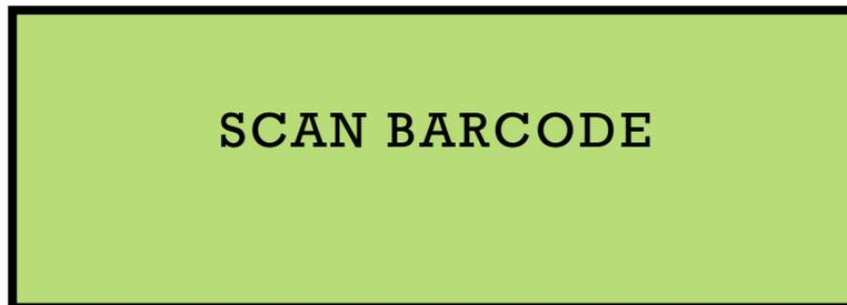
Scan the barcode from the fitting attached to the processor. Remove the Barcode Wand from the protective sheath. While holding the wand at a slight angle, as you would a pencil, position the point slightly to one side of the label and move the wand rapidly across the barcode stopping at a point slightly off the label on the other side.
